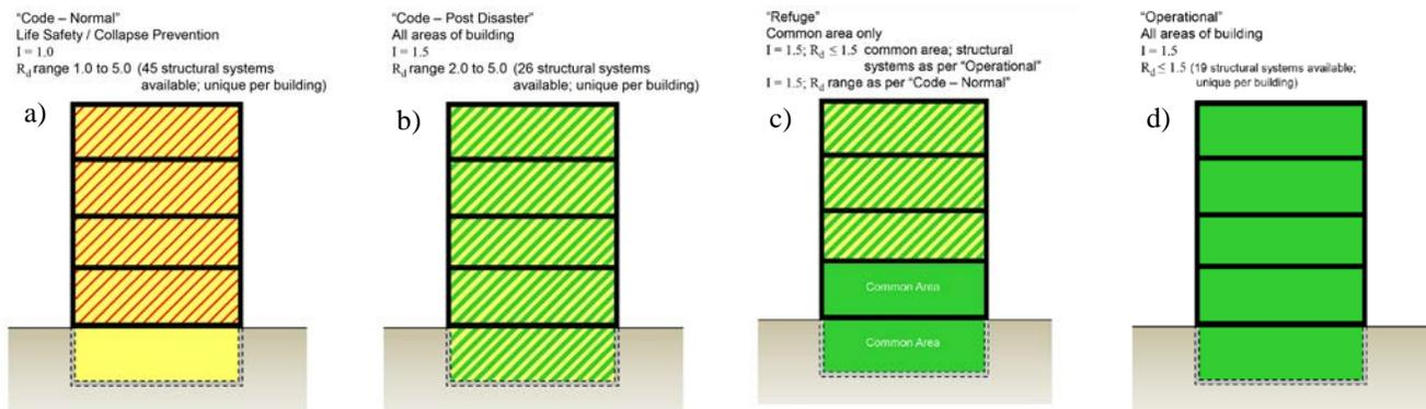
Figure 1. Performance levels: a) Code- Normal, b) Code-Post Disaster, c) Refuge, d) Operational.
